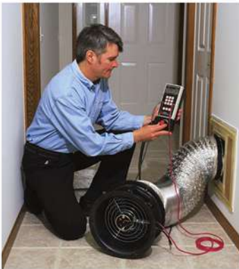
The Minneapolis Duct Blaster® is used to measure the airtightness of duct work.
