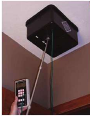
The Exhaust Fan Flow Meter is used to measure exhaust flow through bath fans and other outlets
